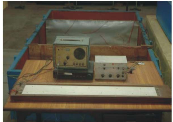
EHDA Model of Jorthang Barrage (Sikkim) showing experimental set-up in Ground Water Laboratory
