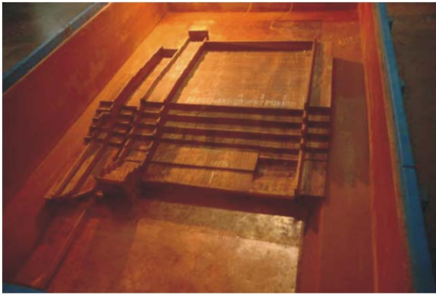
EHDA Model of Jorthang Barrage (Sikkim) showing experimental set-up in Ground Water Laboratory
